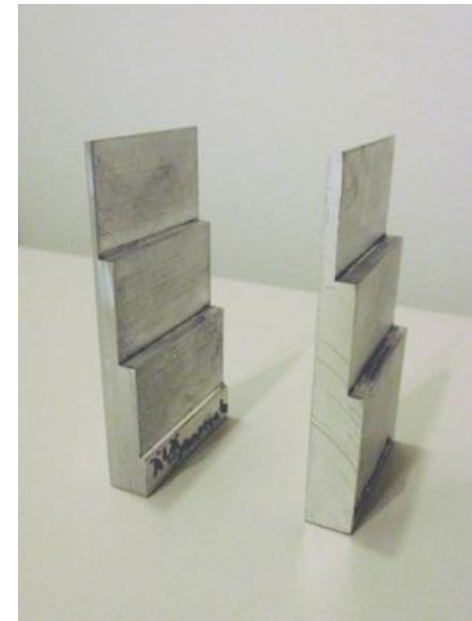
Al plates with different thickness are used in Dynamic Flat-field correction
