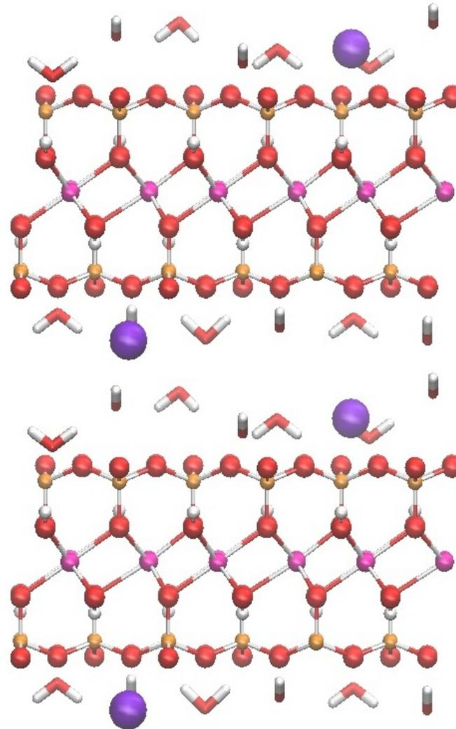
Figure 1: Snapshot of Na-montmorillonite structure (6 unit cells) containing aluminum atoms (pink), silicon (orange), oxygen (red) and hydrogen (white). The interlayer contains water molecules and sodium atoms (purple). Dimension  $16,8\text{\AA} \times 28\text{\AA}$ .
