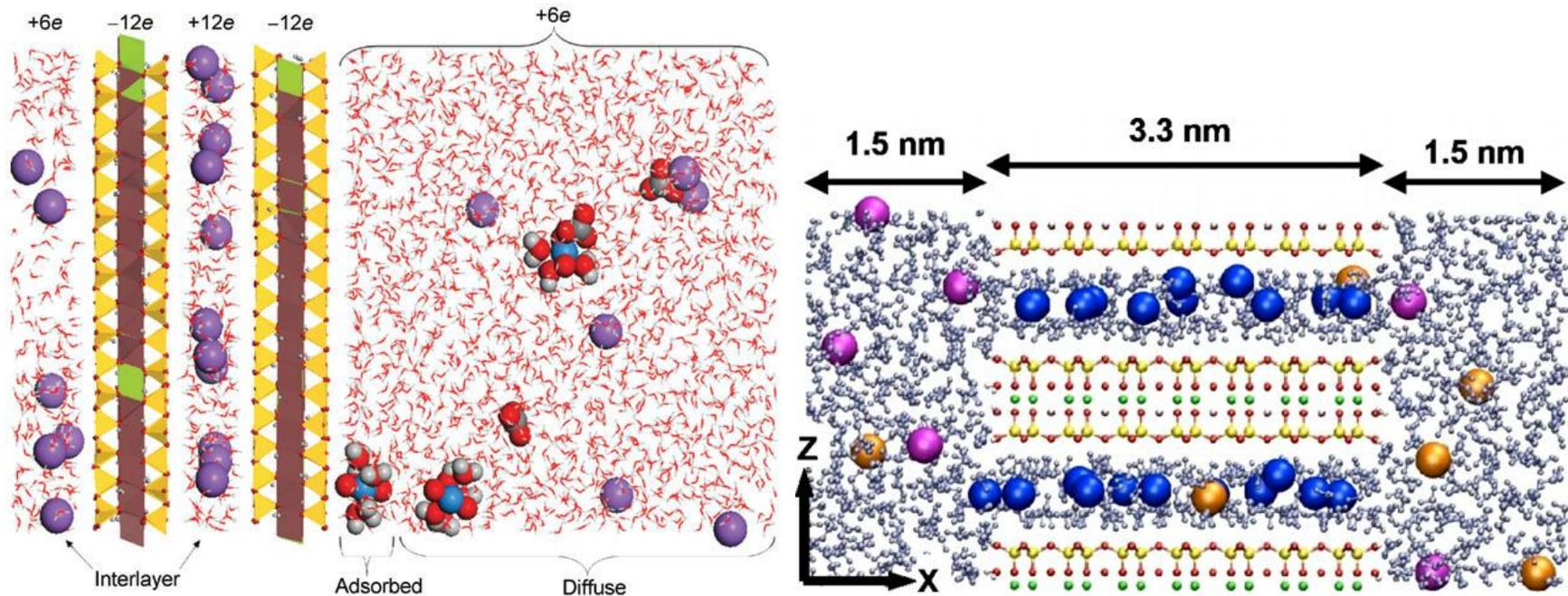
Equilibrium snapshot of an adsorption simulation [1] and simulation box for interlayer/micropore exchange of water/ions [4]
