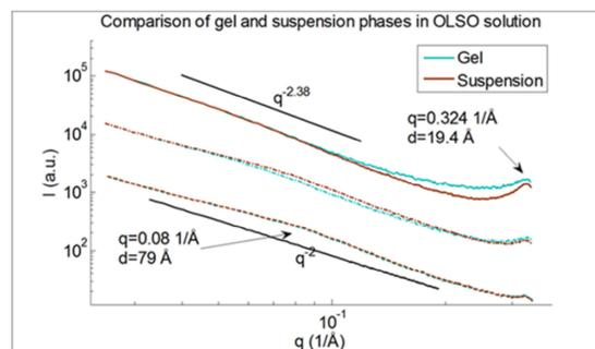
Fig. 3. Comparison of the scattering graphs between the bentonite suspension and gel phase 0.01 M OLSO solution characterized by SAXS [1].
