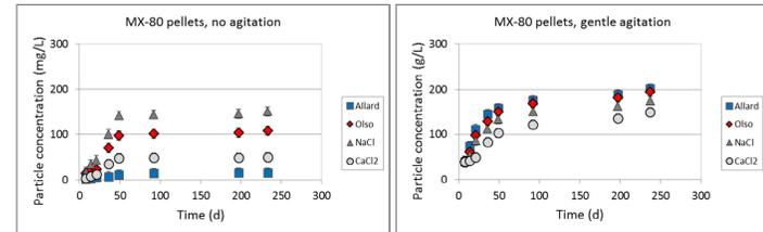
Fig. 6. Mean particle concentration of colloids formed from bentonite pellets in 4.2 mM Allard and 1 mM OLSO, NaCl and CaCl<sub>2</sub> solution without (left) and with gentle agitation (right).
