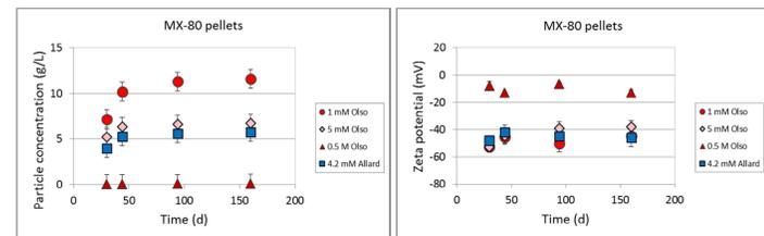
Fig. 8. Mean particle concentration (left) and zeta potential (right) of colloids formed from bentonite pellets in Allard and OLSO solutions with gentle agitation.
