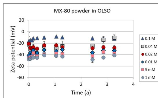
Fig. 5. Mean zeta potential of colloids formed from MX-80 bentonite powder in diluted OLSO reference groundwater.
