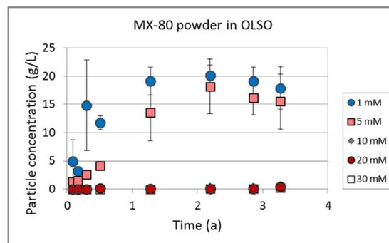
Fig. 4. Mean particle concentration of colloids formed from MX-80 bentonite powder in diluted OLSO reference groundwater.
