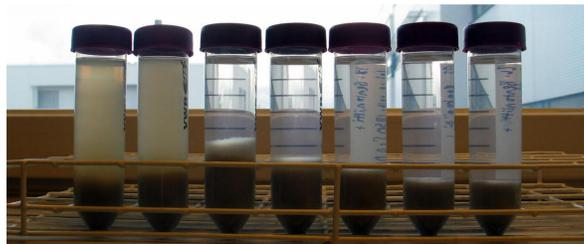
Fig. 2. Formation of bentonite colloids in diluted OLSO, I = 1–30 mM. A thin layer between suspension and colloid fraction is a result of bentonite erosion via gel formation.
