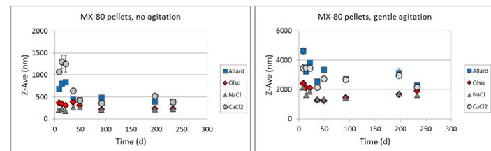
Fig. 7. Mean particle diameter of colloids formed from MX-80 bentonite pellets in 4.2 mM Allard and 1 mM OLSO, NaCl and CaCl<sub>2</sub> solution without (left) and with gentle agitation (right).
