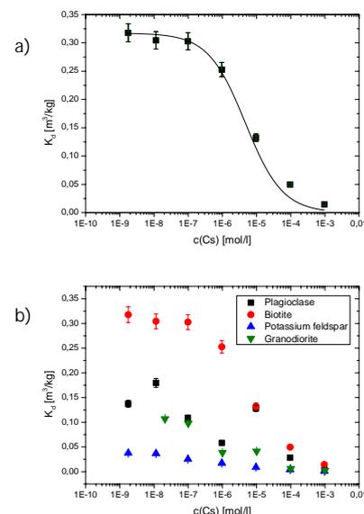
Fig 2. a) The sorption results of caesium on biotite with PHREEQC-modelling. b) The sorption results of caesium on plagioclase, biotite, potassium feldspar and granodiorite
