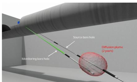
Fig 1. Experimental layout of Phase III of the in-situ test.
