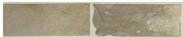
Figure 2. Carbon steel after 3 years of exposure in abiotic (left) and biotic (right) ground water
