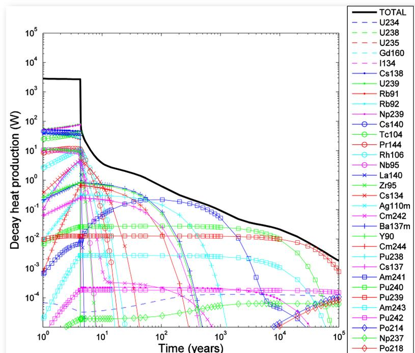
Figure 1: The total and nuclide-wise heat productions of the top-5 decay heat producers. The results are provided in Watts per axial centimetre of the assembly.
